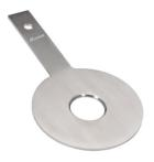
Arrotop's **Square-Edged Orifice Plates** are designed for versatility and precision. They provide accurate measurement of flow rates by creating a differential pressure drop across the orifice. This design is particularly suitable for general applications involving clean fluids, offering excellent repeatability and accuracy. The square-edged orifice is characterized by a sharp edge that appears identical from either direction, making it ideal for bi-directional flow measurement.
