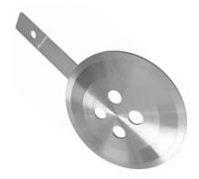
The **Arrotop Multi-Hole Orifice Plate (Model: ARO-MP-005)** features multiple symmetrically placed holes relative to the plate's center. This configuration enhances flow uniformity and reduces turbulence, making it suitable for installations with space constraints. The design ensures effective performance with only 2D upstream and downstream straight lengths, providing improved flow conditioning and reducing noise and pressure drop.
