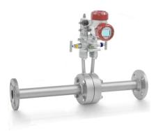
The **Arrotop Integral Orifice Assembly (ARO-OPA-IOA)** is designed to provide accurate and reliable flow measurement for liquids, gases, and steam. This fully integrated flow meter eliminates the need for additional fittings, tubing, valves, adapters, and mounting brackets, thereby reducing welding and installation time. By directly mounting Differential Pressure Transmitters on the orifice assembly, installation costs and potential leak points are significantly reduced.
